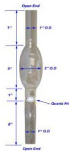
Figure 1. Fluidized bed reactor dimensions.
