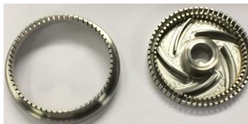
Figure 2 Ytron ZC mixer head stator, on the left, of diameter 0.089 m and rotor, on the right, of diameter 0.095 m
