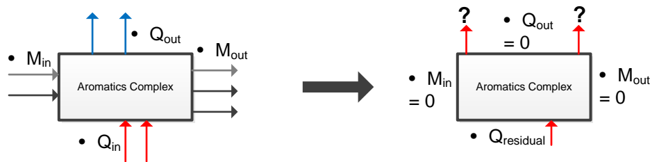
Figure 1. Sketch of the relief load resulting from the residual fired heater duty into the isolated process.
