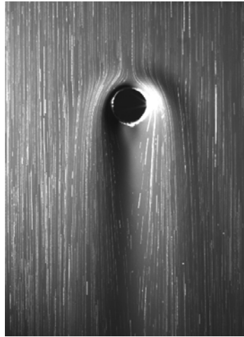
Figure 1. Superimposed image of the thin falling film over a perforated plate seeded with silver coated particles to visualise the free surface streamlines for a low Re flow ( Re = 0.5 ) for silicone oil of \nu = 100 cSt.
