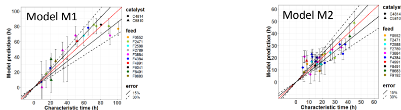
Figure 2. Parity plot with 95% confidence interval for model M1 (left, R^2 = 0.83 ) and model M2 (right, R^2 = 0.66 )
