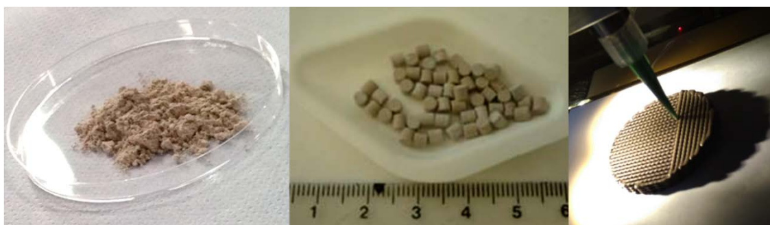
Figure 1. MnNa 2 WO 4 /SiO 2 catalysts for OCM reaction tests; powdered (left), pelletized (middle), 3D printed structures (right)
