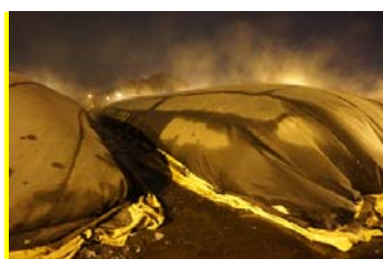
Figure 6. View of piles – vapours do not escape from the isolated edging, but from the membrane surface
