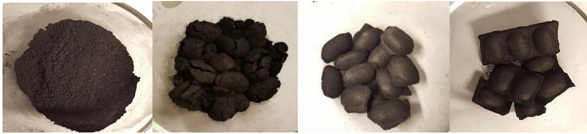
Figure 1: Photo of (a) biocarbon powder, and briquettes made from (b) biocarbon + water 20%, (c) biocarbon + +20% water + 20% alkali lignin and (d) biocarbon + 20% water + 20% starch, after drying at 105 °C for 12 hours
