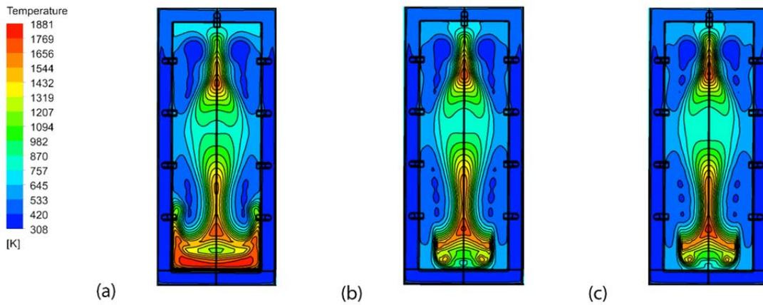
Figure 5: Temperature distribution in the horizontal plane above the fire pit (used also for experimental measurements) predicted with different void fractions of the porous domain: (a)  $\epsilon = 0.4$ ; (b)  $\epsilon = 0.5$ ; (c)  $\epsilon = 0.6$ .
