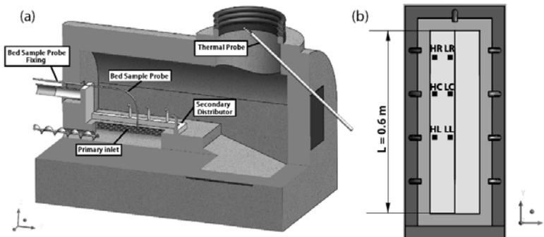
Figure 1: Scheme of the (a) biomass boiler and (b) thermocouples position on the bed (the biomass feeding is from the bottom).
