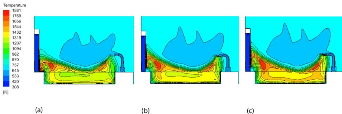
Figure 3: Temperature distribution in the boiler longitudinal mid-plane predicted with different void fractions of the porous domain: (a)  $\epsilon = 0.4$ ; (b)  $\epsilon = 0.5$ ; (c)  $\epsilon = 0.6$ .
