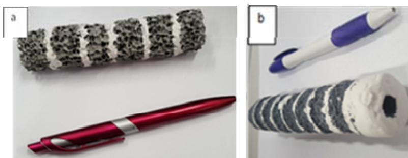
Figure 1: Open-cell foams investigated in this work: (a) 10 ppi OBSIC foam, (b) 65 ppi OBSIC foam.
