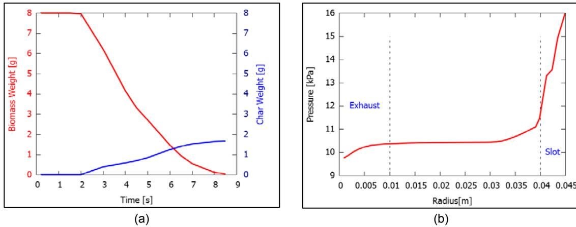
Figure 4: (a) Time-dependent biomass and char weight in the reactor indicating biomass degradation and char formation, (b) Pressure profile in the reactor indicating a low pressure drop of 4-5 kPa across the slots and 1-2 kPa over the solids bed.
