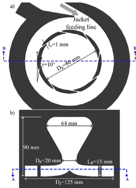
Figure 1 : (a) Top and (b) front views of the Gas-Solid Vortex Reactor highlighting key design features like bottom plate cone and exhaust design (taken from (Gonzalez-Quiroga et al., 2017)).
