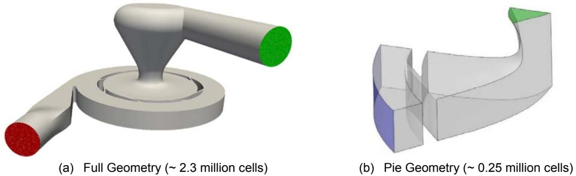
Figure 2: Computationally studied geometries of the GSVR: (a) full geometry including the gas inlet and outlet section. (b) visualized pie section of the geometry containing one slot and part of the gas inlet and outlet section.
