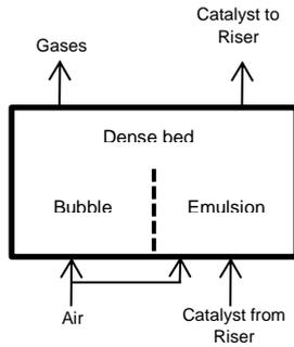
Figure 1: Schematic diagram of the regenerator dense bed model
