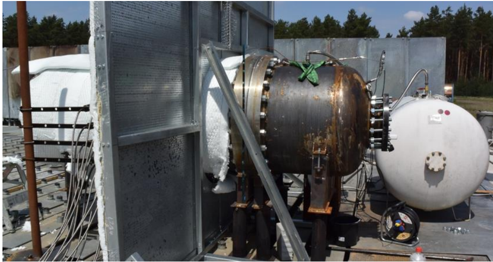
Figure 2: The equipment end showing glass held in position. The supply tank for pressurization of the equipment end is visible to the right.
