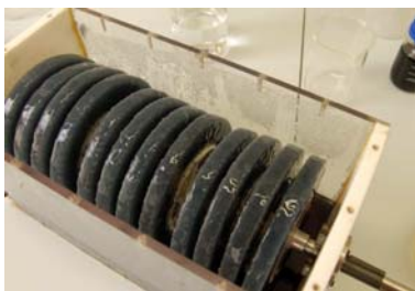
Fig. 2: Rotating disk biofilter with the Irpex lacteus mycelium attached to the Filtren TM discs.
