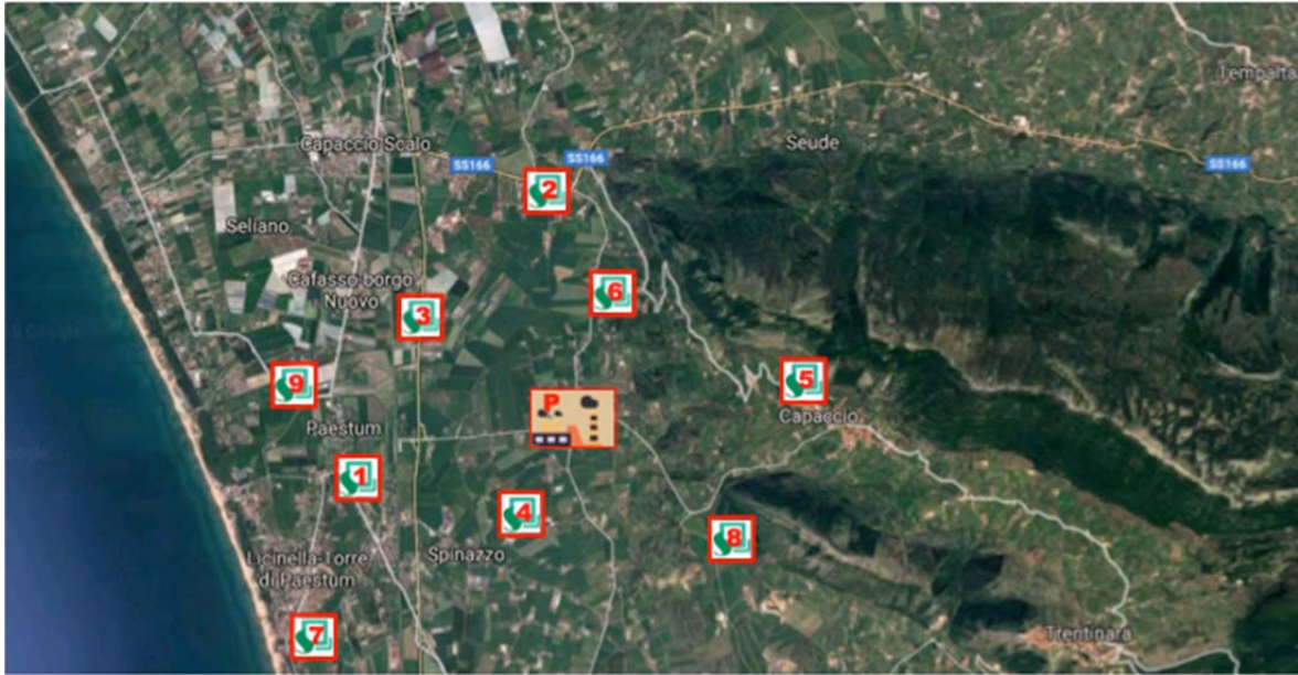
Figure 1: Example of an air quality monitoring network with spatial and temporal high resolution. The sensors are numbered from 1 to 9 and the plant is called P.
