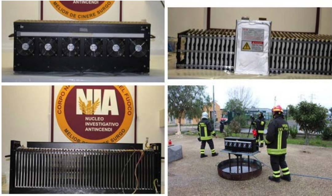
Figure 2 – Battery pack made up of 48 EIG C020 cells.
