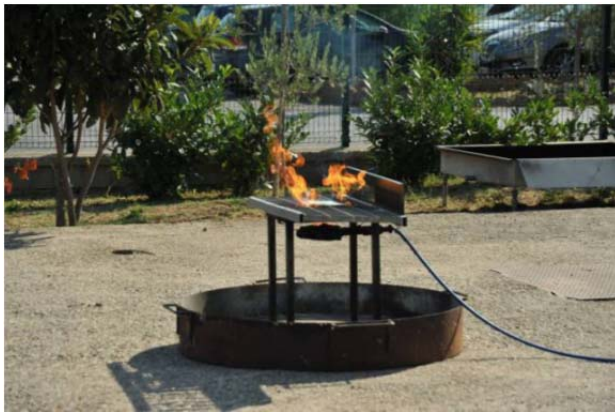
Figure 3 - Experimental setup for thermal abuse tests.
