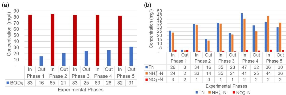
Figure 2: Efficiency of (a) biodegradable compound removal, and (b) Nitrogen compounds removal
