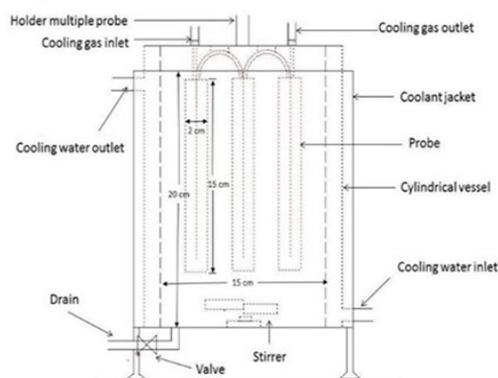
Figure 1: Schematic diagram of multiple probe cryo-concentration system
