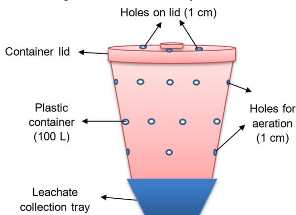
Figure 1: Diagram of the incubation system
