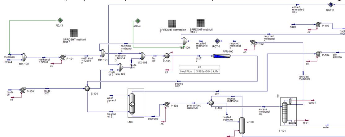
Figure 1: The acid-catalyzed pre-treatment section
