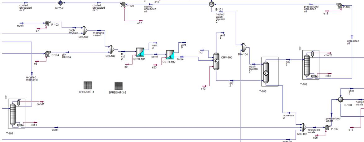
Figure 2: The base-catalyzed trans-esterification section
