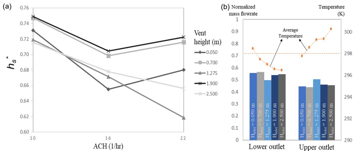
Figure 6: Comparison of (a) normalized sensible heat rate,  $h_s^*$  with different ACHs and vent heights; (b) normalized mass flowrate and temperature of upper and lower outlet for ACH = 10
