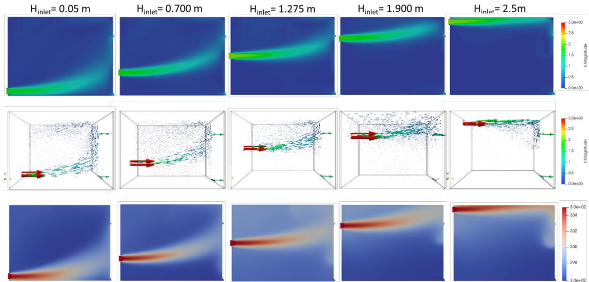
Figure 4: Comparison of velocity contour, velocity vector, and temperature profile of air at the  $xy$ -plane for different vent heights obtained using numerical simulations for  $ACH = 10$ .
