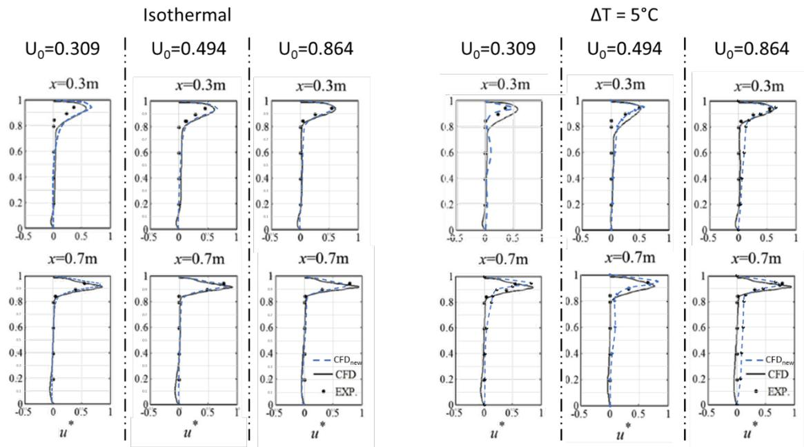
Figure 2: Comparison of  $CFD_{new}$  (isothermal and  $\Delta T_{inlet} = 5\text{ }^{\circ}\text{C}$ ) simulations of normalized  $x$ -velocities ( $u^* = u_x/u_0$ ) with Deng et al. (2018) simulated data and experimental results.
