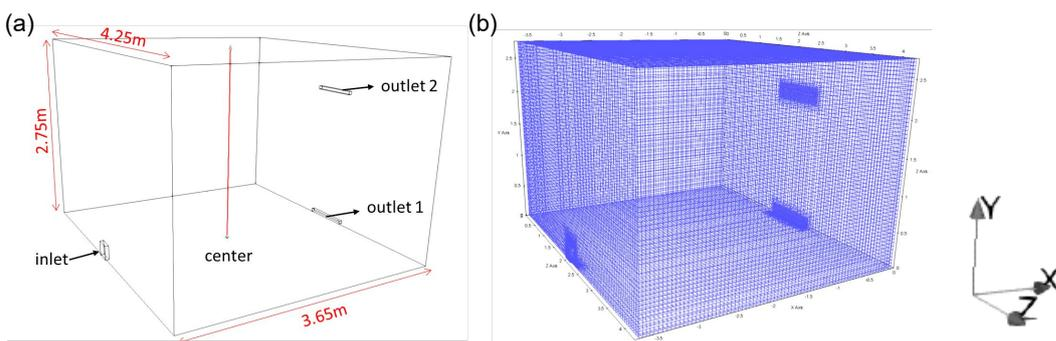
Figure 3: (a) Geometry and (b) mesh of simulated room with fresh air vent height = 0.05 m.
