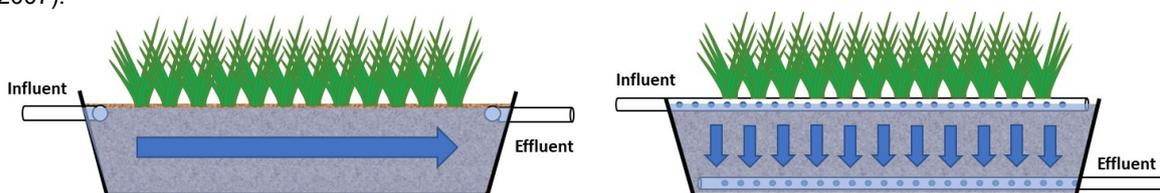
Figure 2: Illustration of horizontal (left) and vertical (right) subsurface-flow wetland
