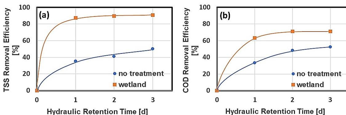
Figure 6: Removal efficiency of (a) TSS and (b) COD in wetland effluent and in control tank
