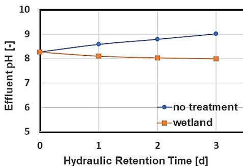
Figure 5: pH changes in wetland effluent and in control tank
