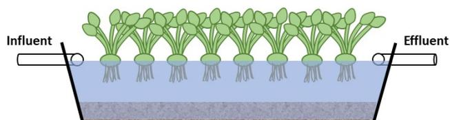
Figure 1: Illustration of surface-flow wetland using floating plants
