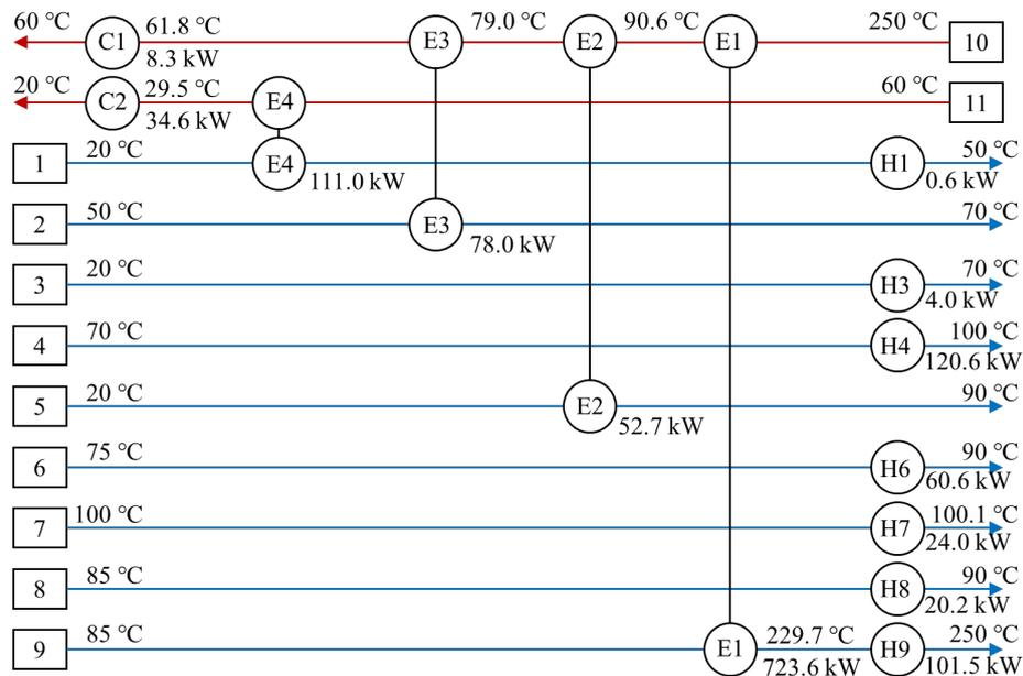
Figure 2: Grid diagram of the HEN after retrofitting using constrained PSO
