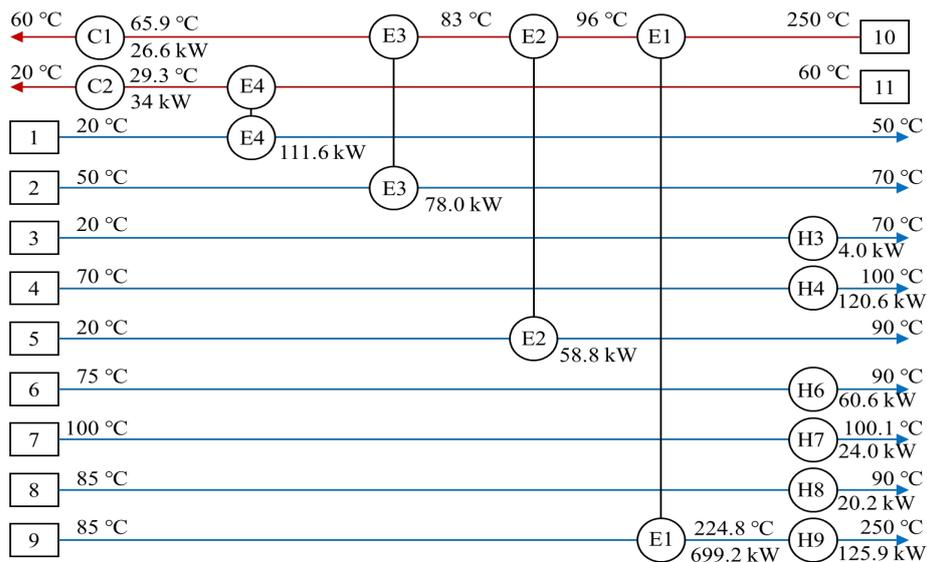
*Figure 1: Grid Diagram of the HEN retrofitted by the graphical method proposed by Lai et al. (2019)*
