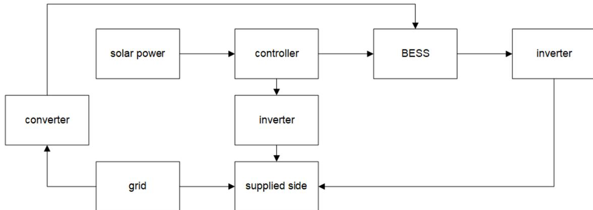
Figure 1: Working Mode of the Solar Power System
