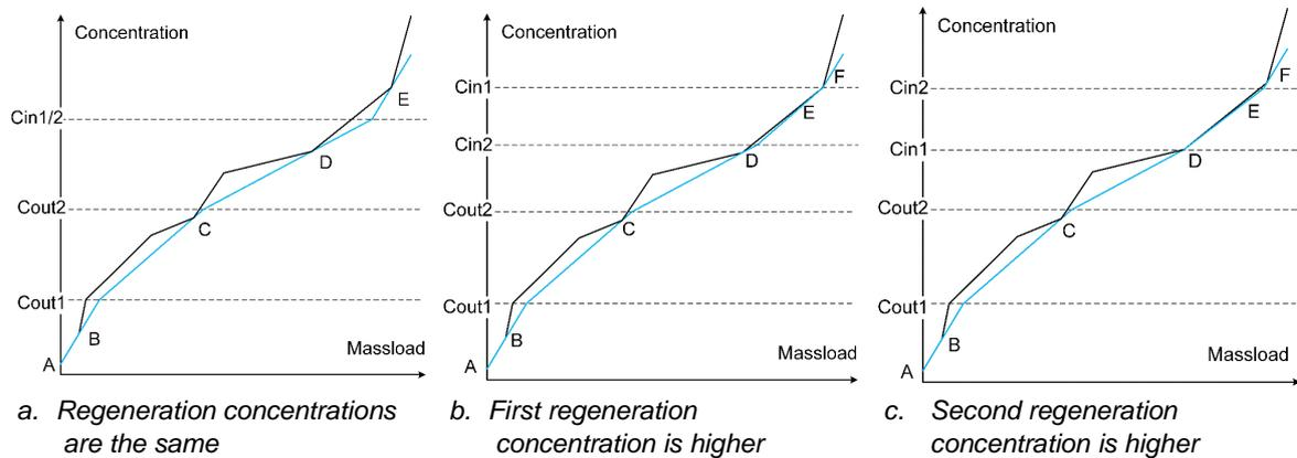
Figure 2: Optimal composite water supply line
