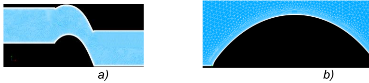
Figure 2: Typical views of the 2D computational grid (~300,000 computational nodes) a) general view, b) enlarged view on the turbine blade suction side
