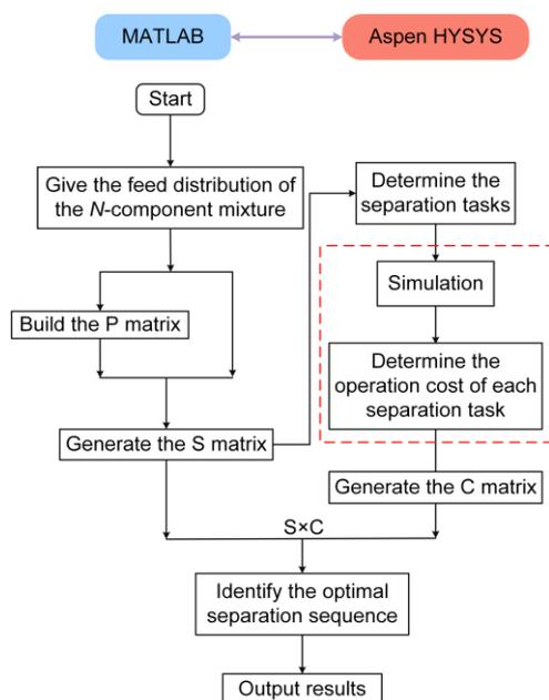
Figure 5: Procedure for automatic identification of the optimal separation sequence
