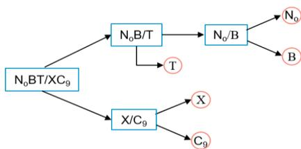
Figure 7: The optimal separation sequence for separating the 5-component hydrocarbon mixture
