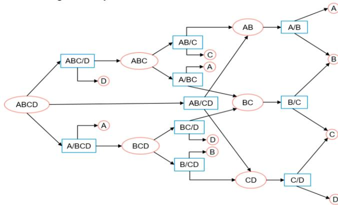
Figure 1: State Task Network Superstructure for a quaternary Mixture
