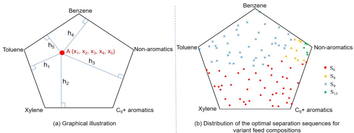
Figure 8: Effects of feed compositions on the optimal separation sequences
