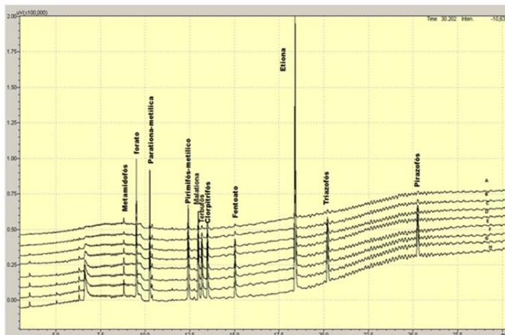
Figure 2: Chromatograms of OP standard solutions at eight different concentrations.
