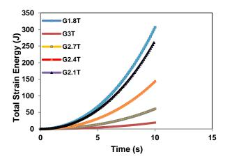
Figure 6: Total strain energy-time response from finite element analysis of G3T, G2.7T, G2.4T, G2.1T and G1.8T, respectively.
