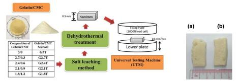
Figure 1: Schematic diagram of salt leaching gelatin/CMC scaffold preparation and experimental test.
