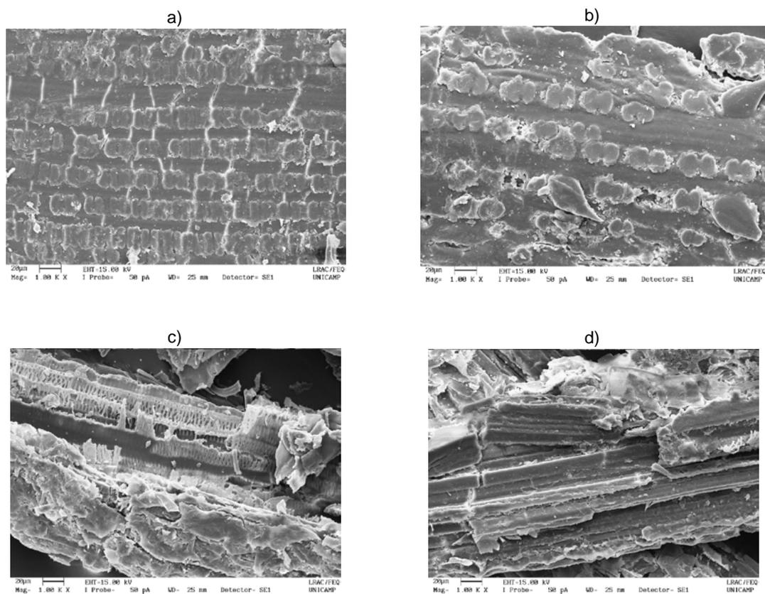
Figure 2. FESEM images of sugarcane straw particles: (a) unextracted; (b) after Soxhlet extraction with hexane; (c) after  $\text{scCO}_2$  extraction without ultrasound and (d) after  $\text{scCO}_2$  extraction without assisted by ultrasound.
