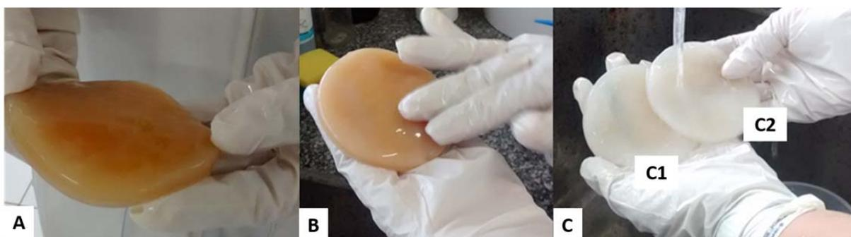
*Figure 1 Macrograph of BC produced after 10 days of static cultivation in HS medium (A) and in alternative medium contend CSL (B). Pellicles after NaOH treatment in, HS medium (C1) and in alternative medium formulated CSL (C2).*
