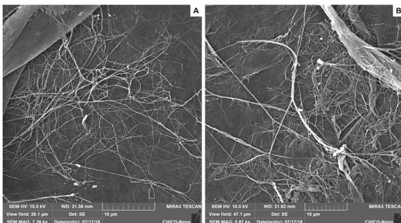
Figure 2 SEM images of BC pellicles obtained after 10 days of fermentation in HS medium (A) and alternative medium formulated with CSL (B).
