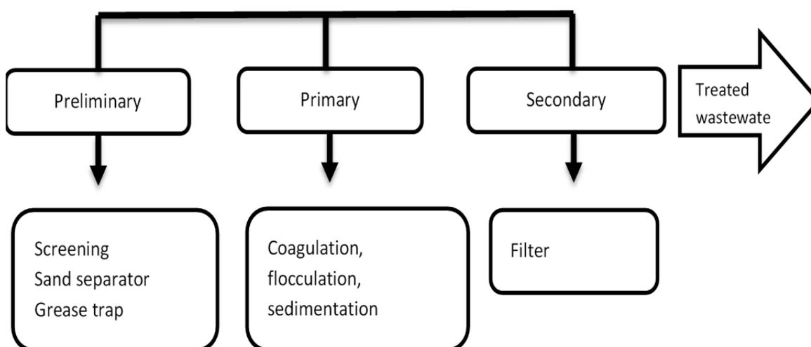
Figure 1: Process 1 Physical-chemical treatment
