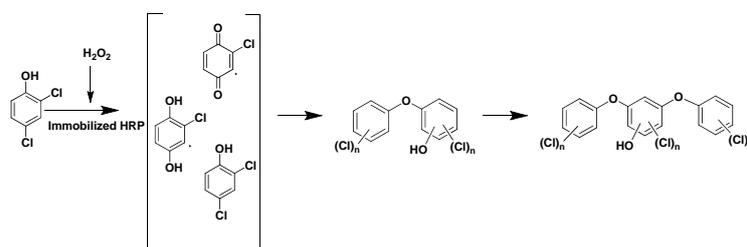
Figure 6. Possible pathways for the oxidative catalytic removal of 2,4-DCP using immobilized HRP.
