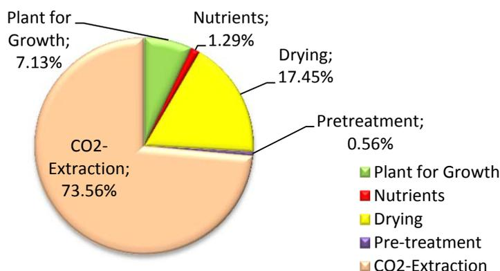
Figure 2. Operating cost index for microalgae growth and EPA extraction via supercritical CO<sub>2</sub> extraction calculated on the basis of the VALUEMAG technology (www.valuemag.eu, 2019).
