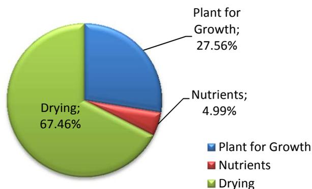
Figure 2. Operating cost index for microalgae growth step calculated on the basis of the VALUEMAG technology (www.valuemag.eu, 2019).
