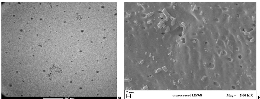
Figure 2: a) TEM image of levan nanoparticles in DMSO and b) SEM image of unprocessed levan.
