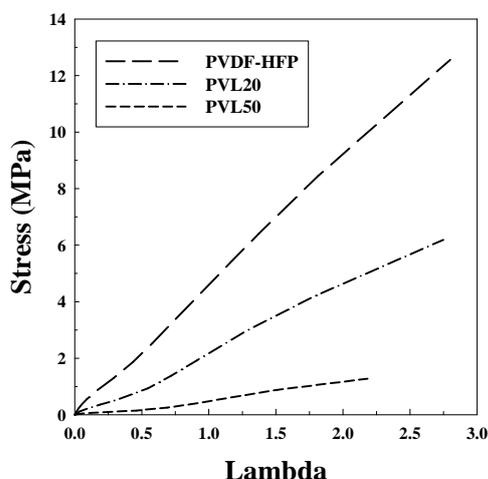
Figure 4: Tensile test for the PVDF-HFP-levan systems: PVDF-HFP, PVL20, PVL50.
