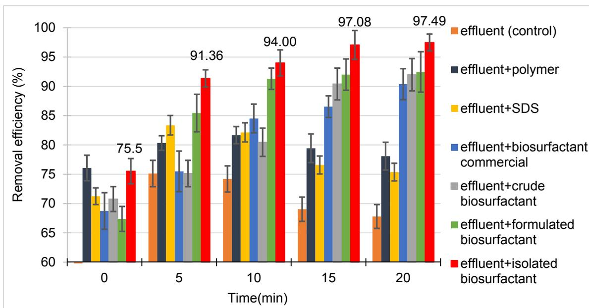
Figure 2 - Results of efficiency of oil removal in industrial effluent by *Pseudomonas cepacia* biosurfactant as collector compared to commercial collectors (SDS, polymer and commercial biosurfactant) associated with the action of microbubbles in the Induced Saturation Tower
