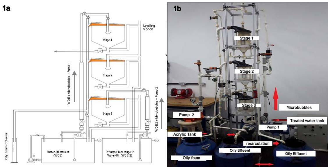
Figure 1 - Bank-scale induced saturation tower. (1a) indicates the flowchart and (1b) actual prototype photo
