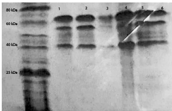
Figure 2: Sodium dodecyl sulfate-polyacrylamide gel electrophoresis (SDS-PAGE) of sunflower protein enzymatic hydrolysates obtained with (1) Pancreatin, (2) Fermgen, (3) Protex 7L, (4) Protex 51 FP, (5) Proteinase T, (6) Protex 40 E. Molecular weight markers (kDa) are indicated on the left.
