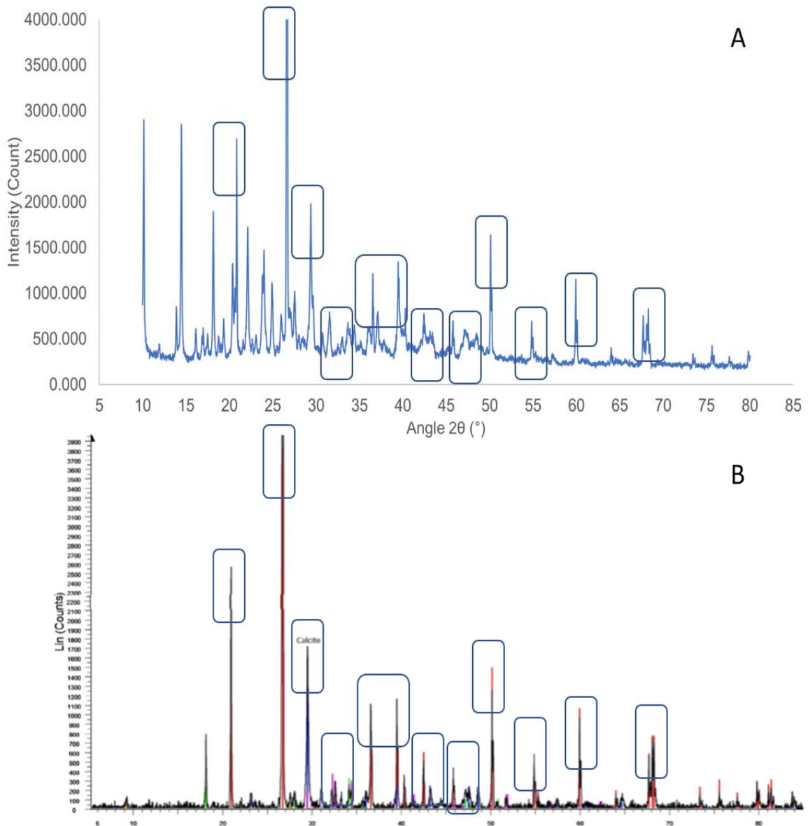
Figure 5: Peaks distribution of crystal formed in: A) biocement produced by *B. cereus*, and B) bioconcrete (Lucas et al., 2018).
