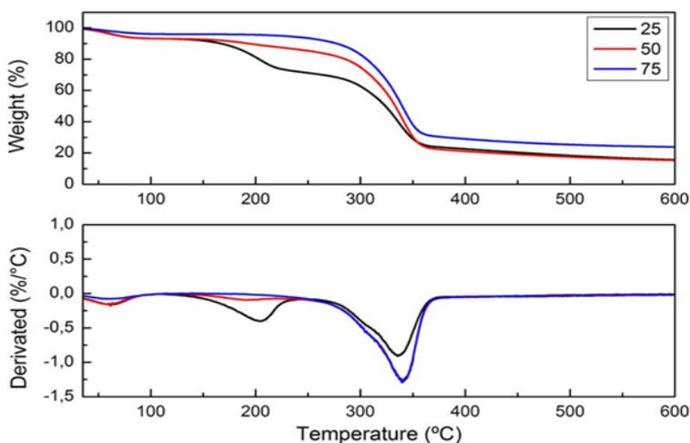
Figure 5 Thermogravimetric analysis graphics of BC75/SCR25, BC50/SCR50, BC25/SCR75 and BC100/SCR0
