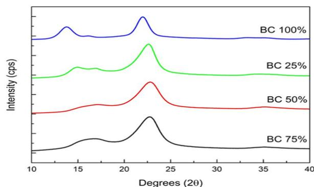
Figure 4 XDR graphics of BC75/SCR25, BC50/SCR50, BC25/SCR75 and BC100/SCR0
