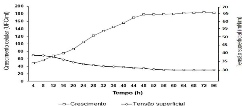
Figure 2: Cell growth and surface tension of *Bacillus invictae* UCP 1617 biosurfactant in 50 L bioreactor over 72h at 175 rpm and 28°C.
