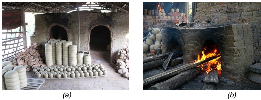
Figure 4: (a) gathering pre-products for combustion; (b) burning wood and coal in the furnace
