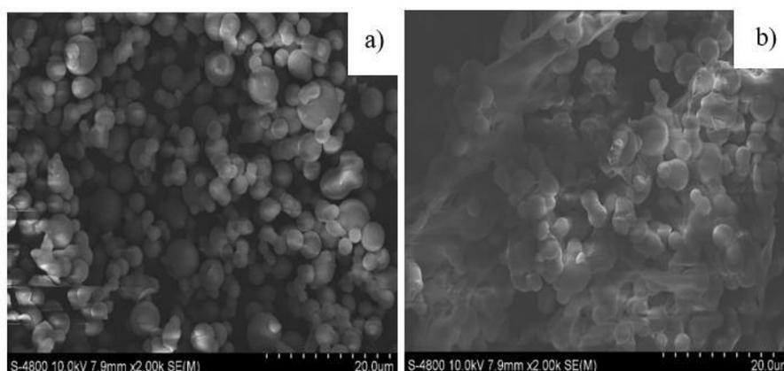
Figure 5: SEM images of the 6 % PTMS/MTMS aerogel (a) without PVA; (b) and after immersion in 1 wt% PVA solution
