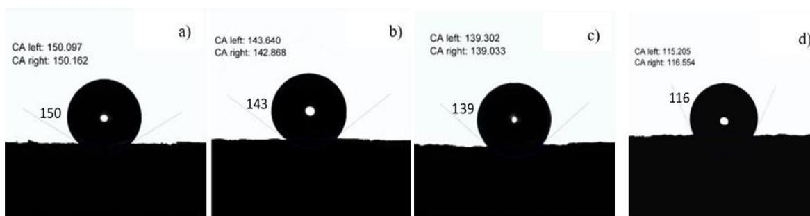
Figure 1: Water contact angles of silica aerogel samples prepared with different PTMS/MTMS molar ratios of (a) 10 %, (b) 6 %, (c) 3 %, and (d) 0 %
