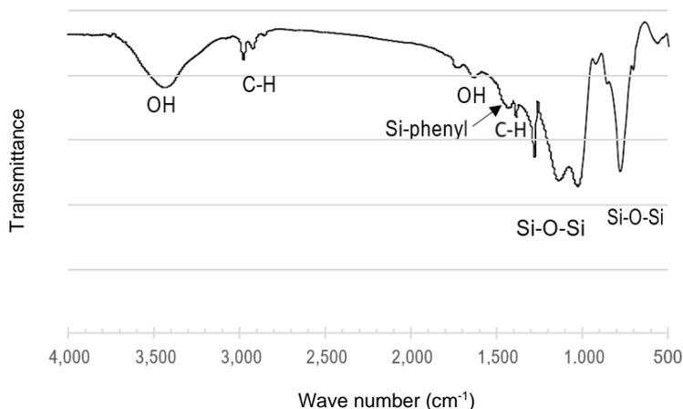
Figure 6: FTIR results of 6 % PTMS/MTMS aerogel immersed in 1 wt% PVA solution
