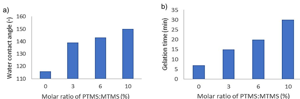
Figure 2: Effect of PTMS/MTMS molar ratio on (a) hydrophobicity of the aerogel samples and (b) gelation time
