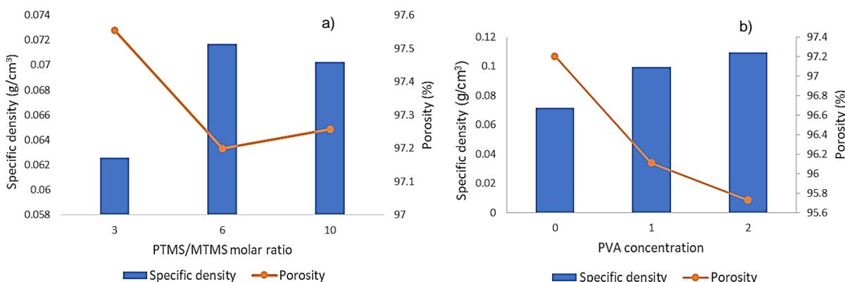
Figure 3: Effect of (a) PTMS/MTMS ratio (%) and (b) PVA concentration (wt%) on the specific density and porosity of aerogels
