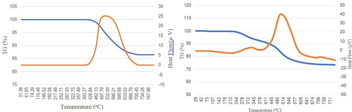
Figure 7: TGA result of 6 % PTMS/MTMS aerogel immersed in (left) 0 and (right) 1 wt% PVA solution
