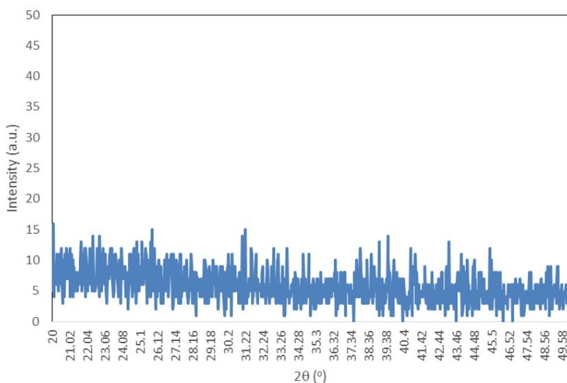
Figure 4: XRD patterns of the 6 % PTMS/MTMS aerogel immersed in 1 wt% PVA solution
