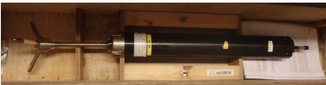
Figure 4: 3D acoustic velocimeter (Vector – Nortek) for horizontal surface current average velocity
