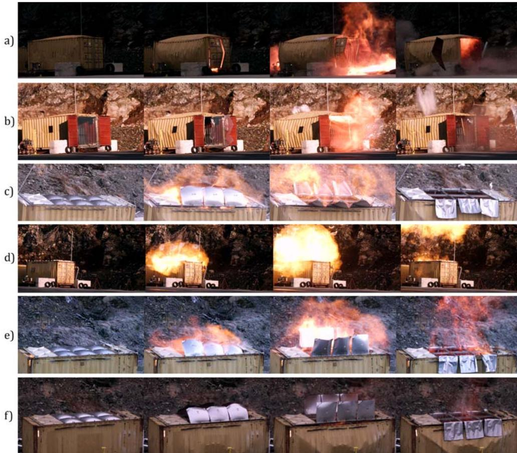
Figure 3: Selected frames from six vented deflagration tests.
