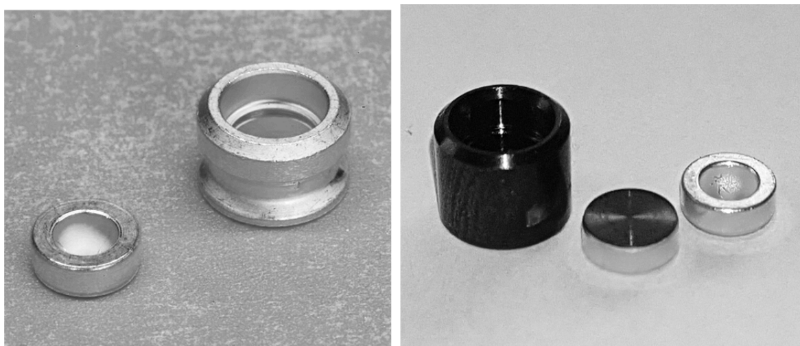
Figure 3: Left: Standard gold-plated crucible M20; right: DLC coated crucible, notice the coating on the inside of the cover
