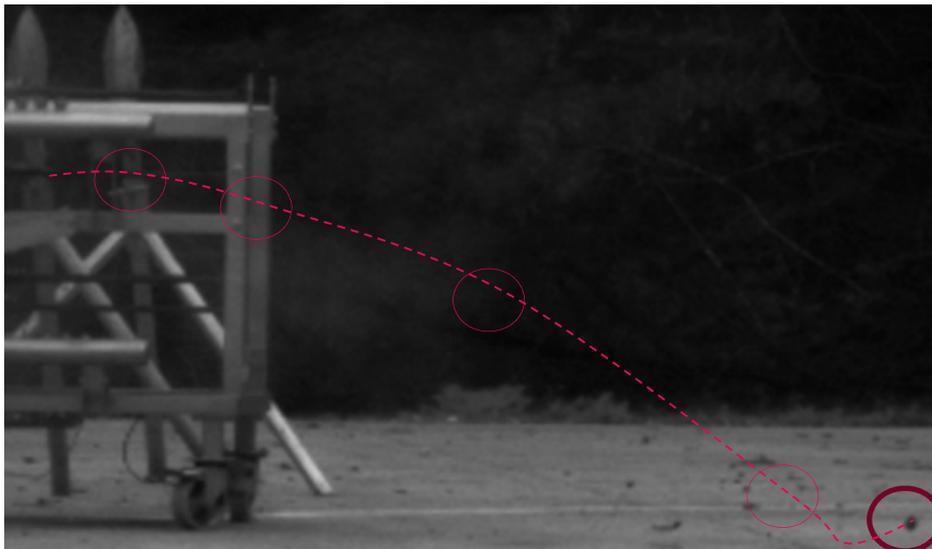
Figure 3. Extracts from the recording of the high-speed camera showing the path of a SiC fragment that allowed the estimation of the kinetic energy of projection.
