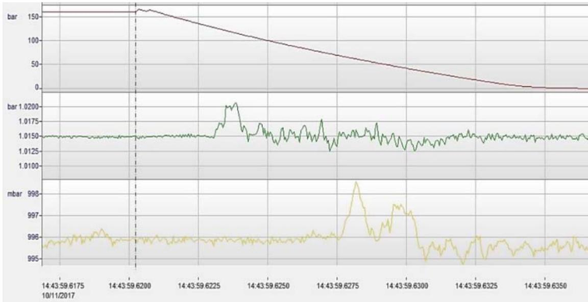
Figure 2: Pressure evolution after bursting: top dark line represents the pressure evolution inside the pressurized SiC plate, the green line is the atmospheric pressure measured at 1m from the centre of the reactor, the yellow line is the pressure measured at 2.5 m from the centre of the reactor.
