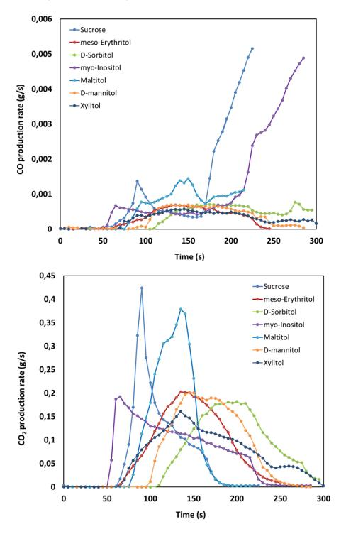
Figure 3: a) (top) CO production and b) (bottom) CO<sub>2</sub> production during Cone Calorimeter Test for sugar alcohols.
