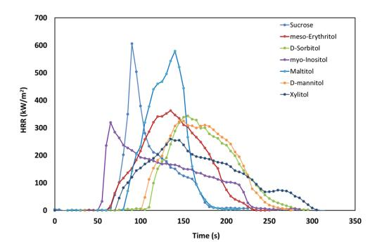
Figure 1: Comparison of HRR development during burning stage for tested compounds (HF = 35 kW/m<sup>2</sup>).
