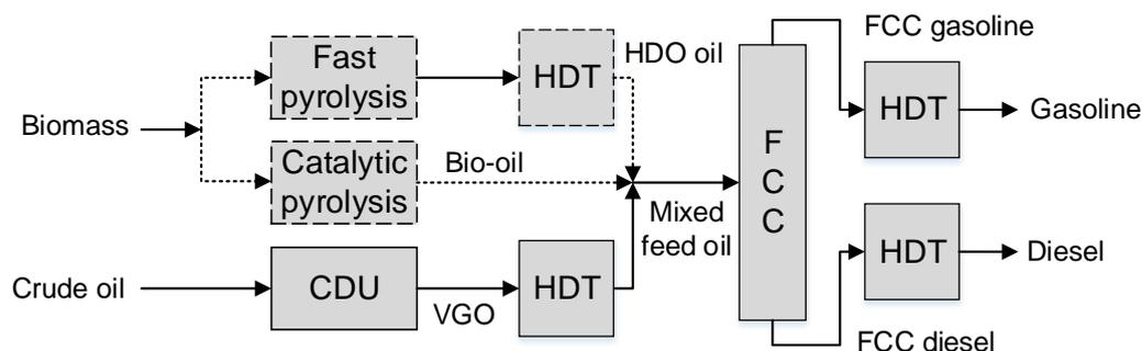
Figure 1: Superstructure of the co-processing of bio-oil and VGO
