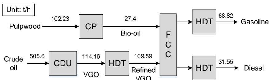
Figure 2: Optimal integration scheme and its main mass balance
