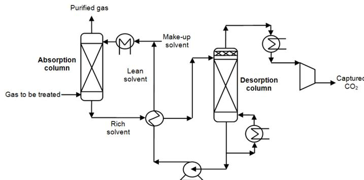
Figure 1: Conceptual design of CO<sub>2</sub> capture unit based on reactive gas-liquid absorption
