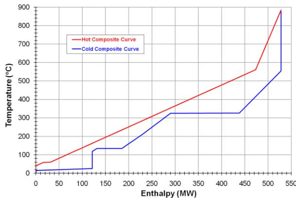
Figure 3: Composite Curves for a super-critical power plant integrated with calcium looping for CO<sub>2</sub> capture
