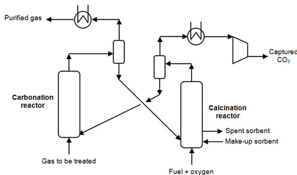
Figure 2: Conceptual design of CO<sub>2</sub> capture unit based on reactive gas-solid system (calcium looping)
