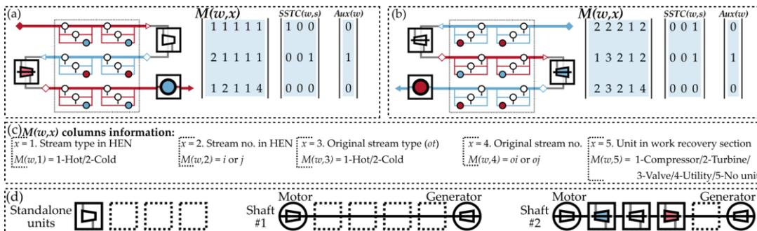
Figure 1:  $M$ ,  $SSTC$  and  $Aux$  variables in (a) example of low-pressure stream with final cooling; (b) example of high-pressure stream with final heating; (c)  $M(w,x)$  columns data and standalone units and multiple shafts in (d).
