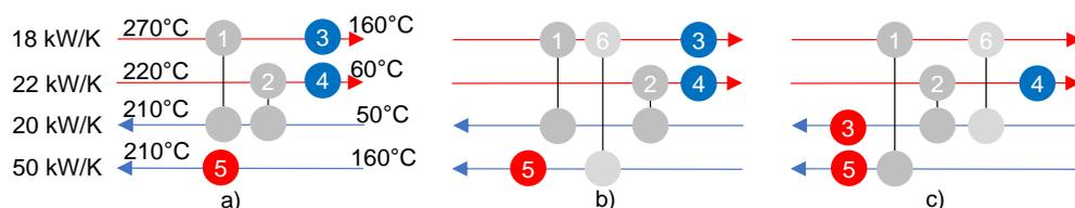
Figure 1: Network structure of a) the motivating example; b) retrofit proposal A; c) retrofit proposal B.
