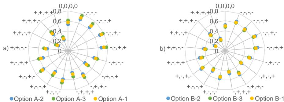
Figure 2: Energy performance ratios at the investigated points of operation for retrofit proposals A (Figure 2a) and B (Figure 2b) and the considered options for flexibility increase according to Tables 3 and 4.
