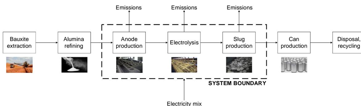
Figure 1: A simplified LCA model for aluminium slug production
