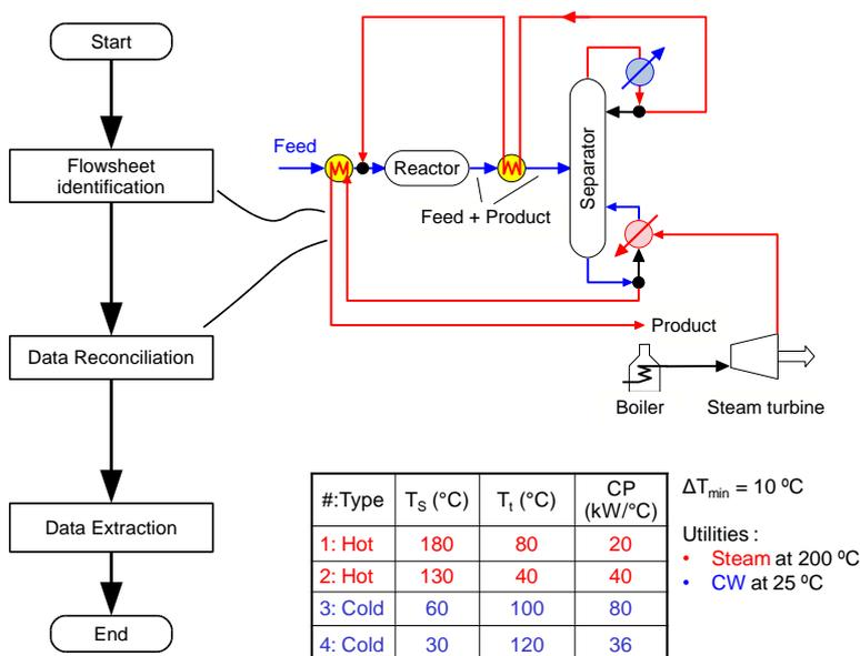
Figure 1. Data acquisition for a process
