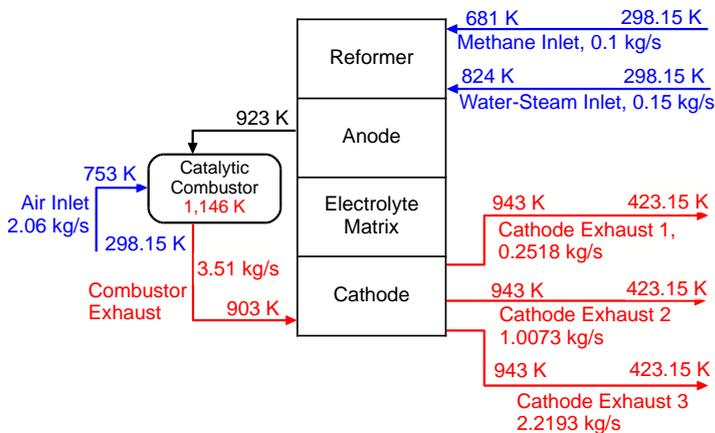
Figure 2. MCFC Flowsheet, adapted from (Varbanov et al., 2006)
