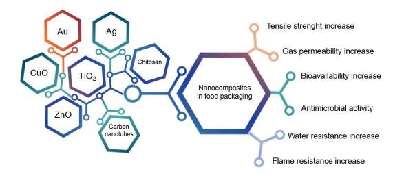
Figure 1: Nanocomposites in food packaging examples and main properties acquired
