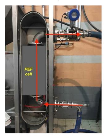
Figure 2: Details of the pulsed electric field (PEF) cell and flow direction
