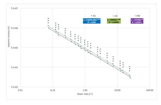
Figure 3: Effect of shear rate on apparent viscosity, plotted in log–log scale, for the two trials (US and PEF), as compared with non-treated olive paste. Different letters denote significant differences (analysis of variance (ANOVA) and honestly significant difference (HSD) test, p < 0.05).
