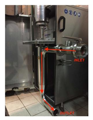
Figure 1: Ultrasound (US) machine, detail of cell flow, US probe and flow direction.
